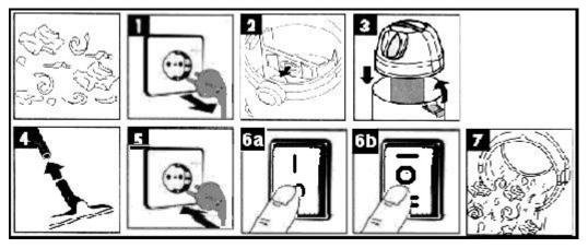
Unplug before change filter (Figure 1), then take out the bag and empty the dust or replace the bag. Slip the dust bag onto the socket(figure 2) for dry vacuum-cleaning.
